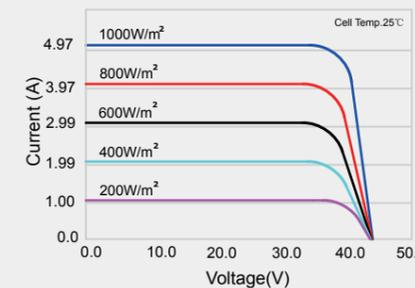
**I-V Curves of module SY-S180W at various cell temperatures**
