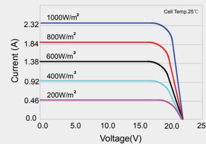
I-V Curves of module SY-S40W at various cell temperatures
